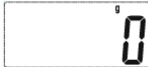
8. If there is no operation, the backlight will be off after about 30s, and the scale will turn off automatically after about another 30s. Or you can touch and hold the On/Off/Tare button for about 2s to turn off it.
