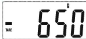
7. When it displays the negative weight, touch the On/Off/Tare button again, it will clear to zero
