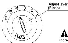
The rinse aid dispenser has six or four settings. Always start with the dispenser set on "4". If spots and poor drying are a problem, increase the amount of rinse aid dispensed by removing the dispenser lid and rotating the dial to "5". If the dishes still are not drying properly or are show spots, adjust the dial to the next higher lever until your dishes are spot-free. The recommended setting is "4". (Factory value is "4".)
