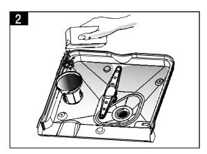
Remove the lower basket and then unscrew and remove the cap from the salt container.
